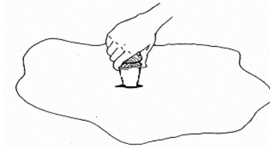
Figure 2. Wood Plug Installation.
